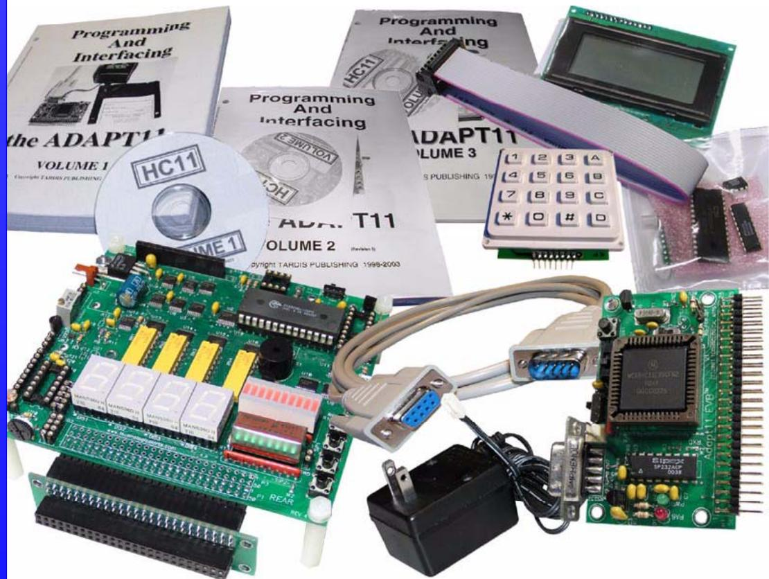
Technological Arts and Tardis Publishing have joined forces to put together a complete low-cost Learning System for the Freescale 68HC11. Courseware is based on Adapt11EVBU and Adapt11 Memory-mapped Interface Board (MIB) to provide complete training in microcontroller interfacing and programming concepts for one of the most prevalent 8-bit microcontrollers in the world. This courseware is currently used in programs offered by Seneca College, Toronto, Canada and Eastern Michigan University.
