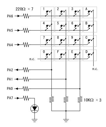
The top six  $220\Omega$  resistors serve the purpose to protect the microcontroller in case of wiring error, and the one tied to PA7 is a current limiting resistor for the LED. The  $10K\Omega$  resistors pull down to zero volts the matrix keypad column wires when no pushbutton is pressed.
