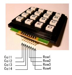
Each of the keypad pushbuttons activates a normally-open switch. Pressing a pushbutton closes a switch between the corresponding row and column wires. For example, pressing button 8 connects Row3 to Col2. The matrix arrangement reduces the number of wires required to interface with these switches from 17 (one per switch plus a common) to 8.
