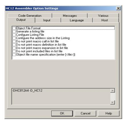
Under Output Tab Select Checked marked the Object File Format and Generate a listing file.
