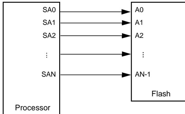
**Figure 3. Byte Address Processor Connected to x8-only Flash**
